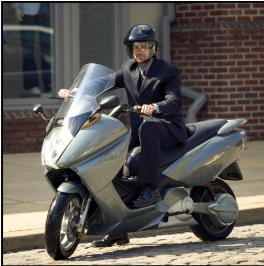
The Vectrix Maxi-Scooter has a top speed of 100 km/h, and a range of over 110 km per charge using nickel-metal-hydrate (NiMH) batteries. It is available for sale in the U.S., Europe and Australia.
