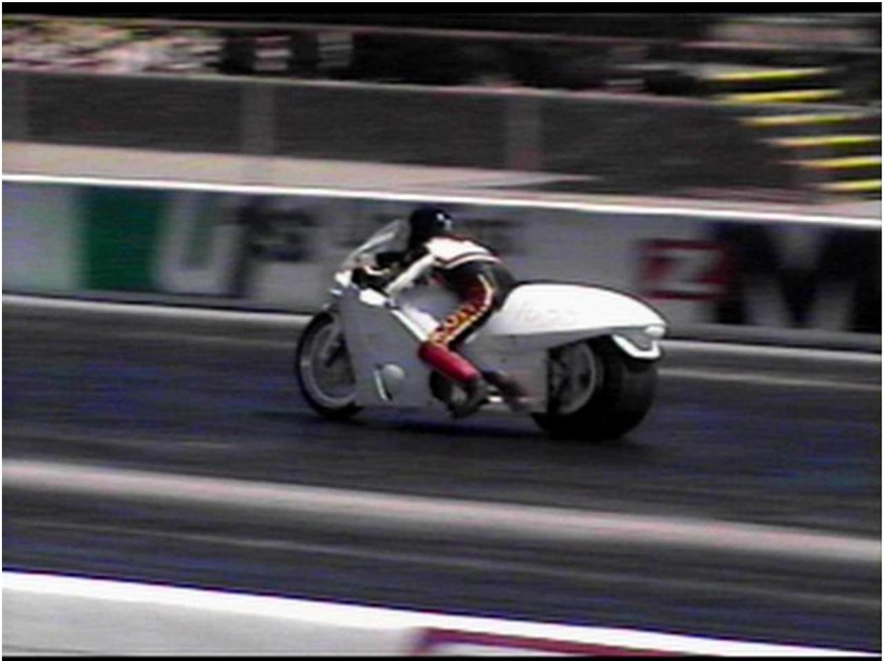
The Killcycle, pictured above, is an electric drag racing motorcycle. It covers the quarter-mile in 9.450 seconds, and hits the trap at 152.07 mph—243 km/h.
